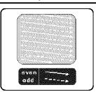
In interlaced-scan video, a frame consists of two interlaced fields (odd and even), where each field contains every other horizontal line in the frame. The odd field of alternating lines is displayed first, and then the even field is displayed to fill in the alternating gaps left by the odd field to form a single frame. One frame, displayed every 1/30th of a second, contains two interfaced fields, thus a total of 60 fields are displayed every 1/60th of a second.
